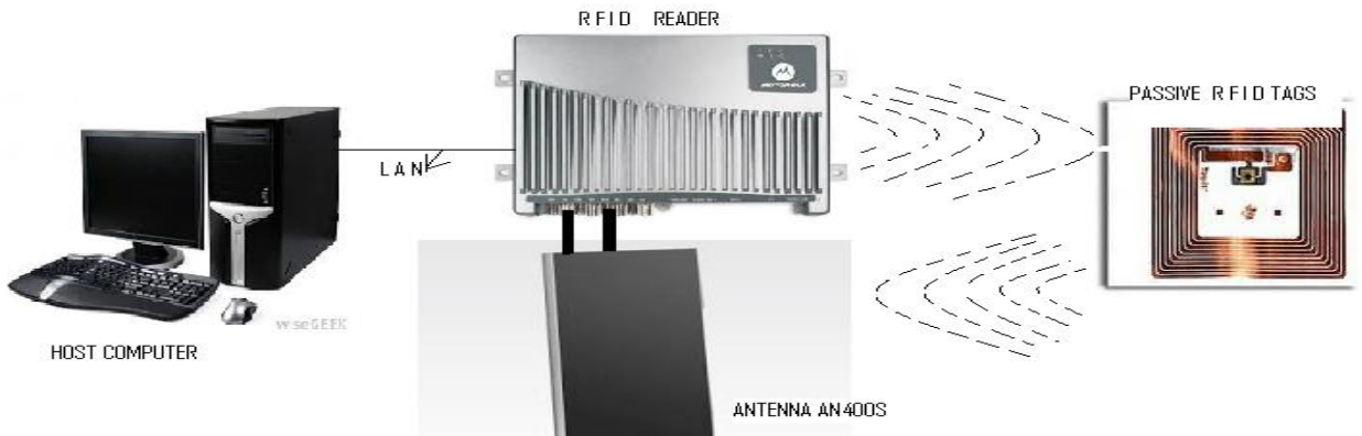
Fig. 3. Antenna-RFID Network Model
